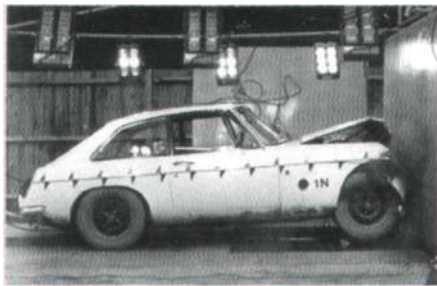
B GT at point of 30mph + impact taken at MIRA.
