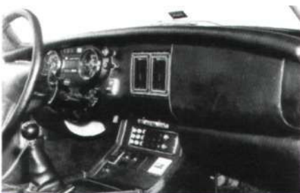
SSVI Airbag & Knee protection mounting collapsing column- impact sensor-under knee roll & British Leyland Automatic start "Test" unit.
