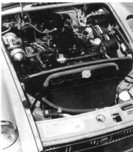
SSVI Underbonnet – showing suspension control and roll/ride levelling units.
