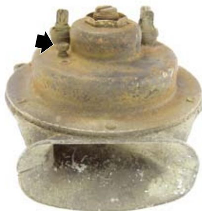
Figure 17.2. A typical pre-1975 horn. The adjustment screw is arrowed.
