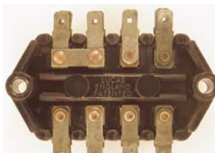
Figure 7.7. If the fuse block connector blades can be easily rocked from side to side they will not make good electrical connection to the fuse clip. They can be tightened by supporting the top side of the rivet and tapping the bottom side with a nail punch.
